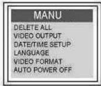
Press MENU to enter function selection. Press UP or DOWN to move cursor to make selection and press OK to enter the selected function.
